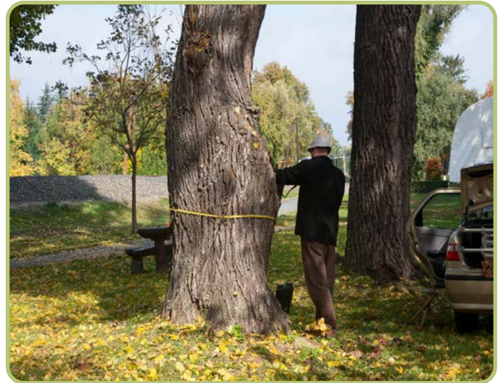
► Image: Acoustic tomography tree scan
